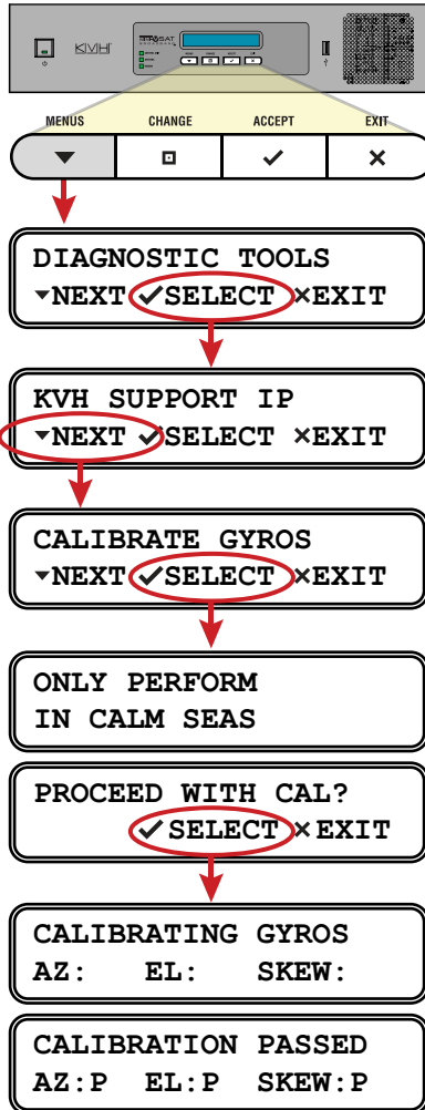
Figure 9-13 Calibrating the Gyros
